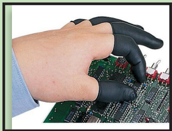
Finger Stalls: A safer way to handle electronics
