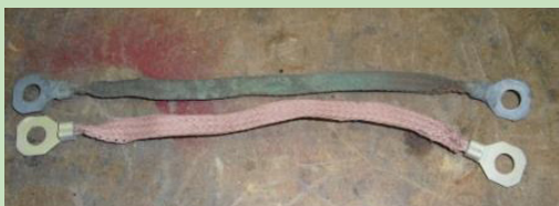
Shiny copper braid quickly corrodes once it's exposed to the elements.
