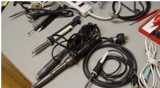
Soldering irons come in many styles and heat ranges. A 25 to 40 watt iron does most jobs.
